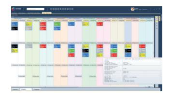
You can check machine capacity during planning. You can automatically set the time for conflicted planning records. You can prevent planning of the processes for the wrong machines by creating process machine groups.
